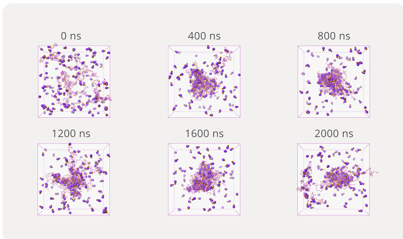
Figure 1: Snapshots at different times from the late-stage dissolution simulation of the IBP/SLP system in water at pH 6.8. The empty space in the box is occupied by water. It's rendered transparent for better visibility of the polymer and drug molecules.
