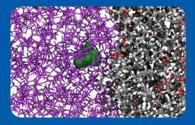
Snapshot obtained from MD simulation displaying the imminent migration of a monomer (methyl methacrylate, in green) from its polymer matrix (polymethyl methacrylate, in purple) towards a palmitic acid formulation.
